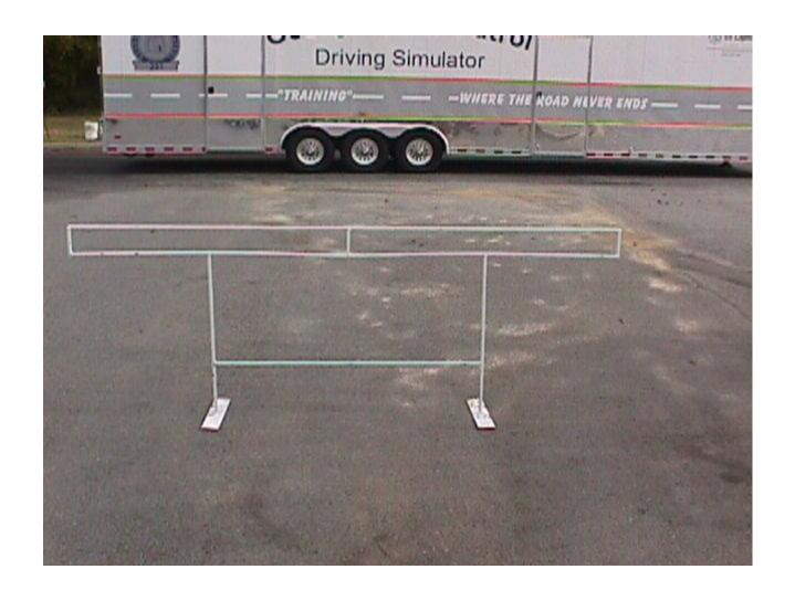
1/2" STEEL TUBING (FEET) 1/8" FLAT STEEL
